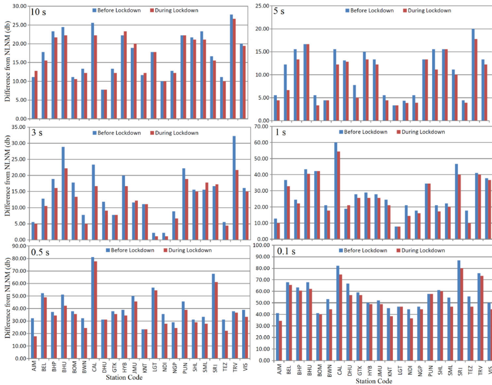
Figure 3. Histograms at various periods (10 s, 5 s, 3 s, 1 s, 0.5 s and 0.1 s) show variations in seismic noise with reference to the new LNM at different seismic stations before and during lockdown.
